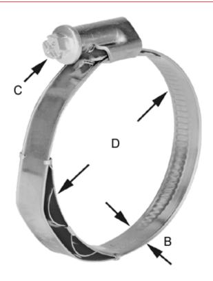
C (screw type) = C7 Diameter D = 16-28 Width B = 9
